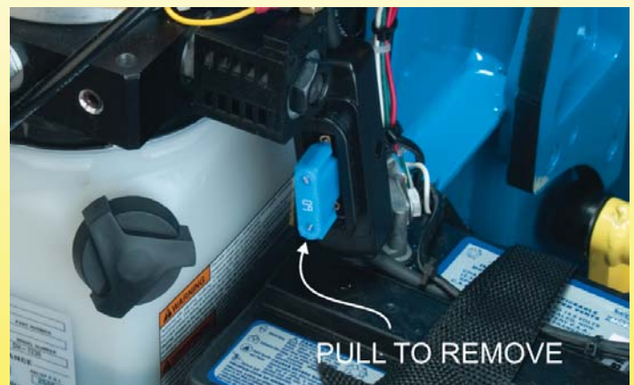
Figure 25 Main Power Fuse
