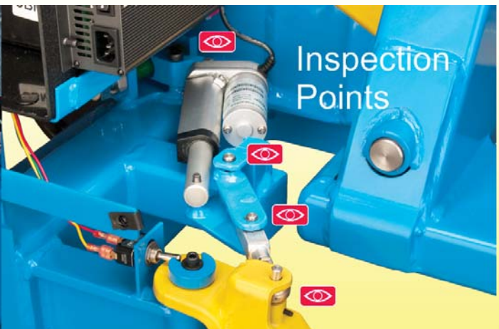
Figure 31 Outrigger Inspection Points
