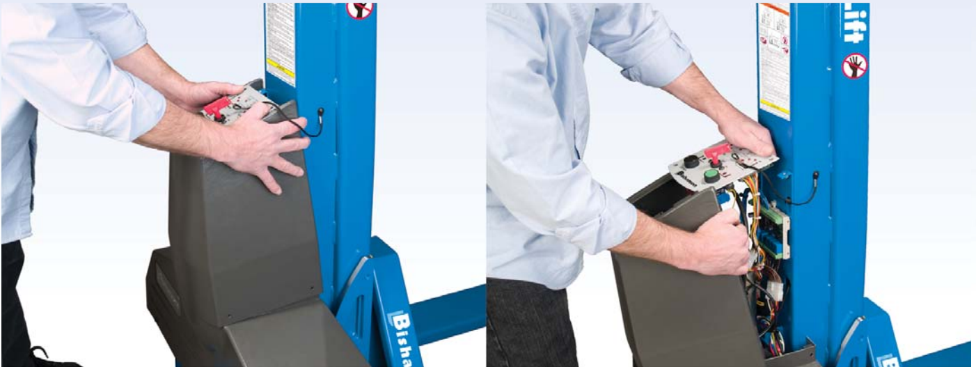
Figure 23 Upper Console Cover Removal
