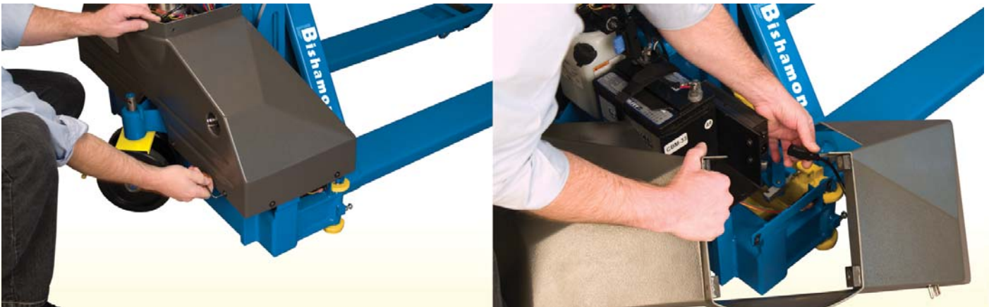
Figure 24 Lower Battery Cover Removal
