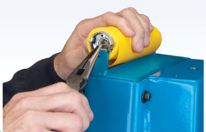
Figure 27 Roller Installation
