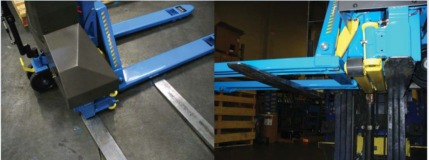
Figure 5 Forklift Lift Points
