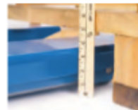
Forks lower to 3.3 in. for optimal clearance under skids.
